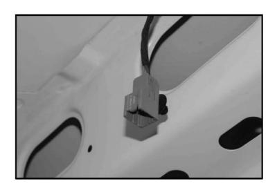
Plug in pigtail to camera connector and then locate this connector in the header of the rear of the truck.
